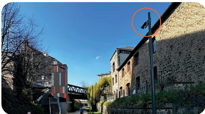
CITIX-AI can be installed on a high point to allow counting over a large area. It counts, classifies and gives the direction of travel of pedestrians, cyclists, mopeds, cars, trucks and buses. You can find and analyse the data on Eco-Visio.
