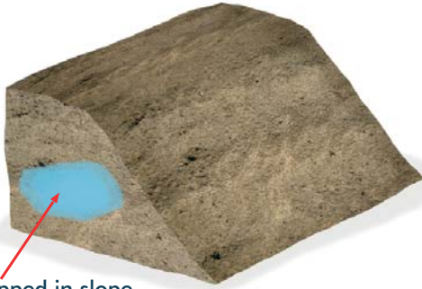
Water trapped in slope
